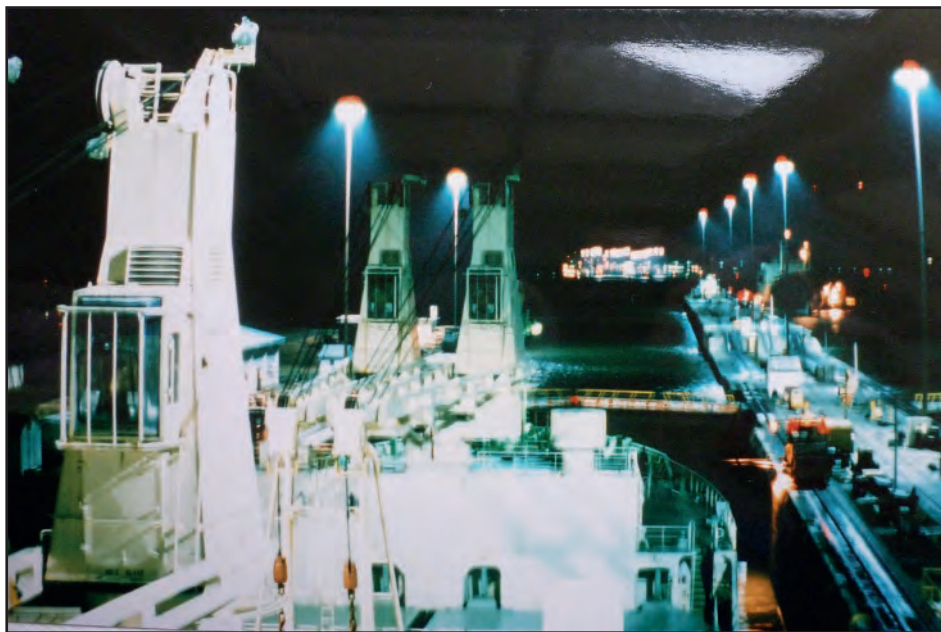
Image 4: Vessel at the Panama Canal with guiding trains at the side and lock gates in front.
