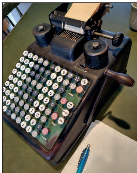
Burroughs Portable Adding Machine, 10kg in weight. Built around 1930, in use in the Farm Surveys Section up to decimalisation in 1971. In those days they built them to last. Note the red keys for farthings!
