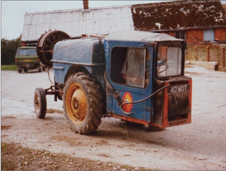
Ferris's self-propelled hop sprayer: it was his first invention for the family farm ...
