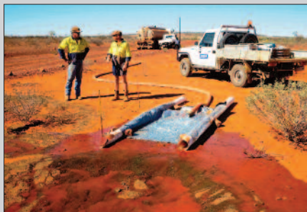
A battered-back and Stonewall treated gully head was subjected to 10,00l of simulated runoff.
